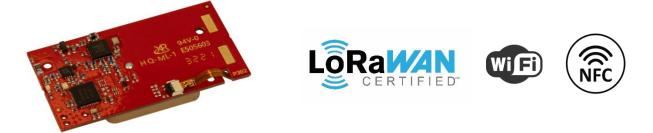
The TM-2016 / P3B2 is a product line member of KCS' advanced TraceME track and trace modules. It is designed for tracking and tracing a variety of IoT assets, targeting industrial, smart cities, transportation and logistics.
