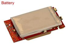
The module is equipped with a non-rechargeable battery.
